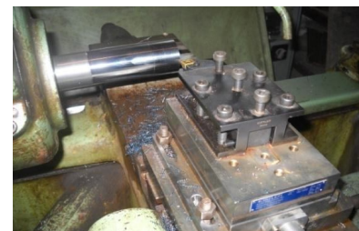
Figure 1: The work piece and tool setup
